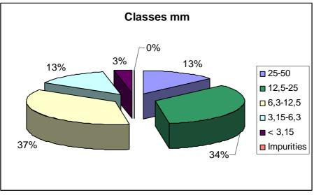
**Graphic1**: (%) break down of the material chopped in the different dimensional classes.
