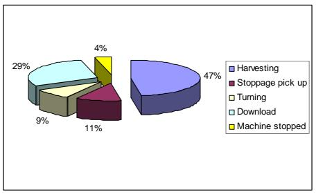
**Graphic 2**: (%) break down of the work yard phases. The unproductive times resulted of about 14,5%, it must be attributed for the major part to the pick-up system stoppage.
